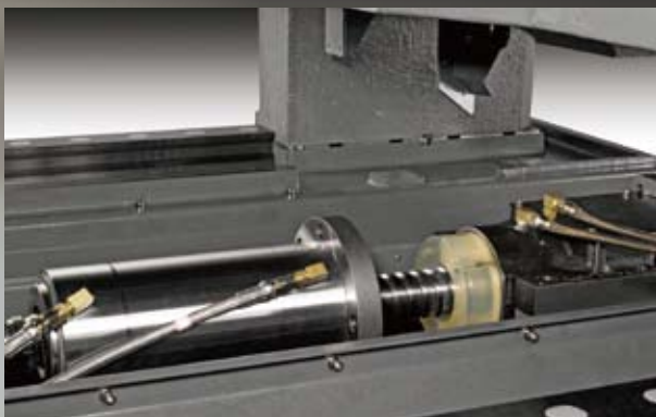
■ Circulated Sleeve Cooling
